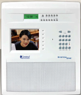
Traditional Master Station sized to retro-fit existing Valet and Electron master installations. Fascia: 320(w) x 390(h) Recess: 270(w) x 325(h) x 75(d)mm
