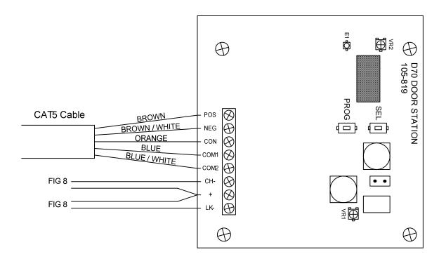
**NOTE:** Plug pack can be wired into "POS" & "NEG" at any station. See "Maximum Length For Cable Runs" in relation to Plug Pack location.
