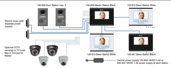
Door station/s to Room Station/s minimum wiring requirements: 4 core screened cable (100-960) + RG59 coax, star wired to master. \*In some installations the 100-958 Video Door Station may have audio feedback when used with a weathershield. A simple modification to the microphone gain is available - please ask when ordering.
